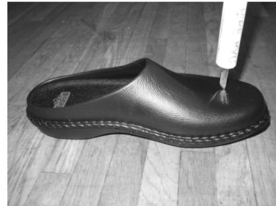
Figure 3. Falling scalpel not able to penetrate through the new rubber shoe.
